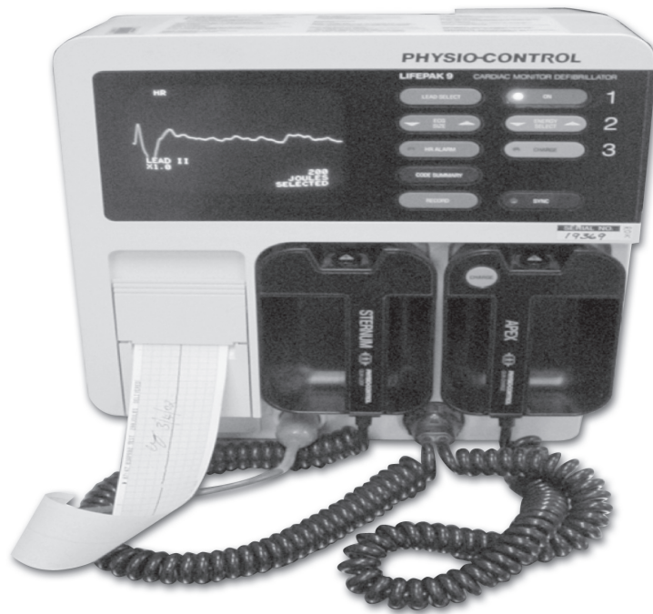
Figure 2.3: Manual or Conventional defibrillator (Lifepak 9) with paddles.
