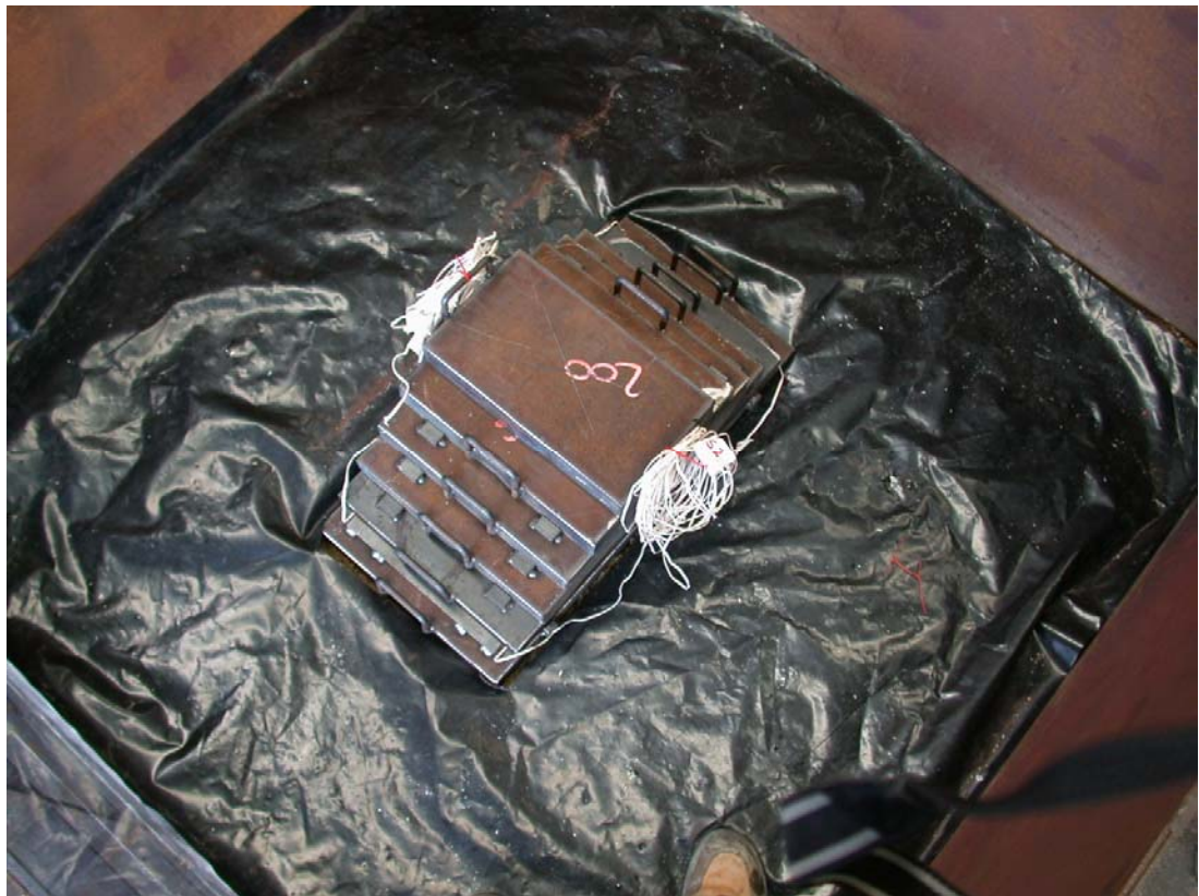
Figure 6.18 Covered top surface hindering moisture evaporation
