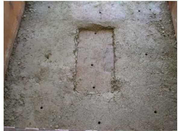
(b) Drilled holes layout ready for taking measurements of density
