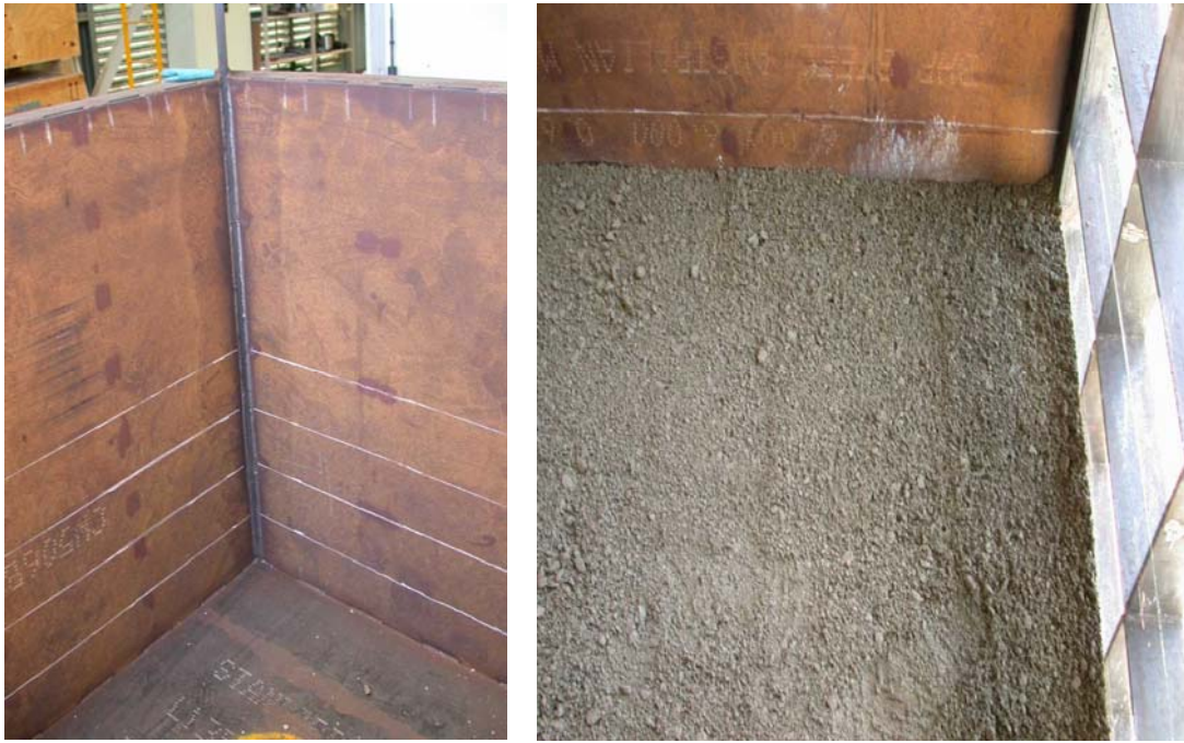
Figure 6.14 150mm thick layers marked on the walls of the box and a levelled material layer ready for compaction
