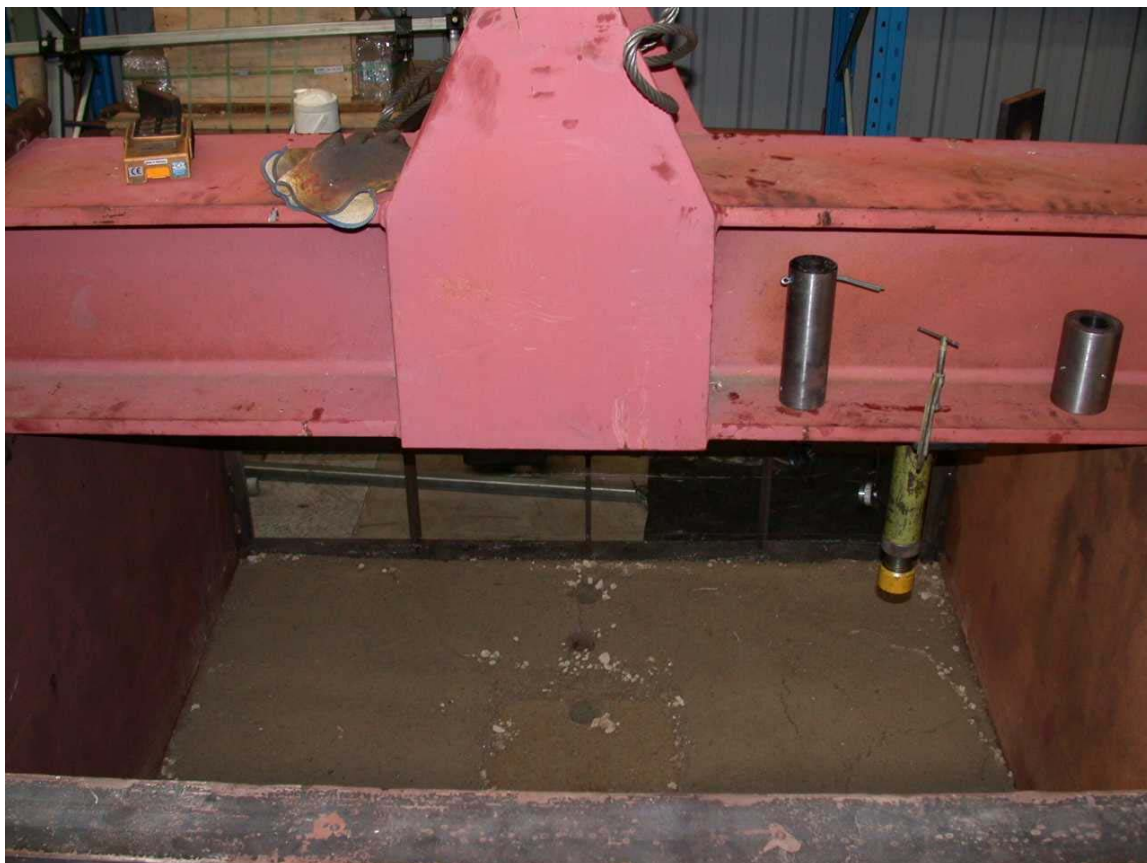
Figure 6.23 Obtaining core samples along the centre line of the specimen using a 50mm diameter sampler
