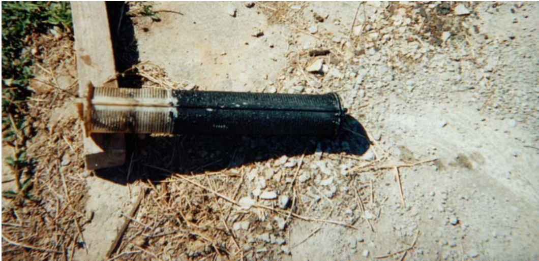
Figure 2.2 In-line filter after 3 months of operation
