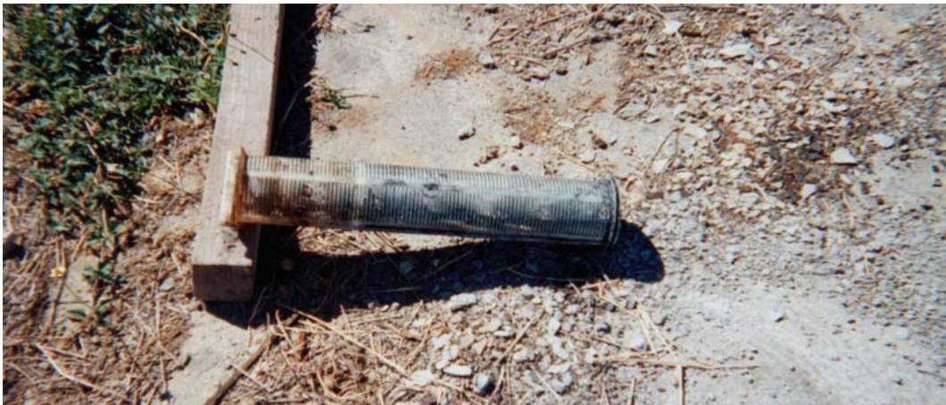
Figure 2.3 In-line filter after maintenance wash
