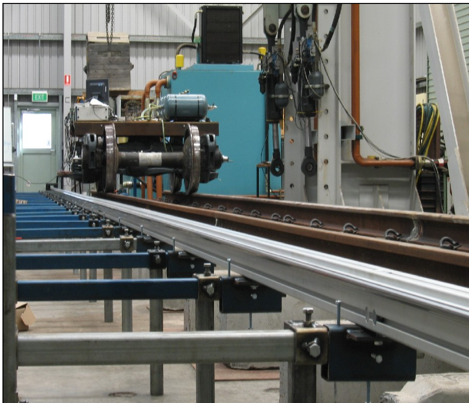
Figure 6.27. Instrumented Bogie with DAQ ready for commissioning
