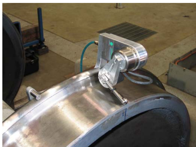
Figure 6.19. MiniProf tool for measuring the wheel profile
