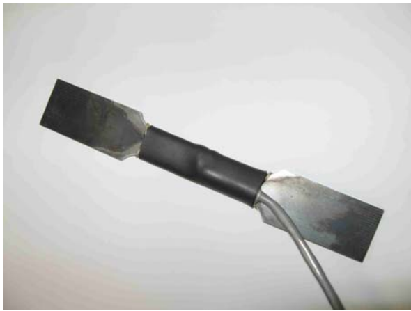
(a) part of the hanger with strain gauge
