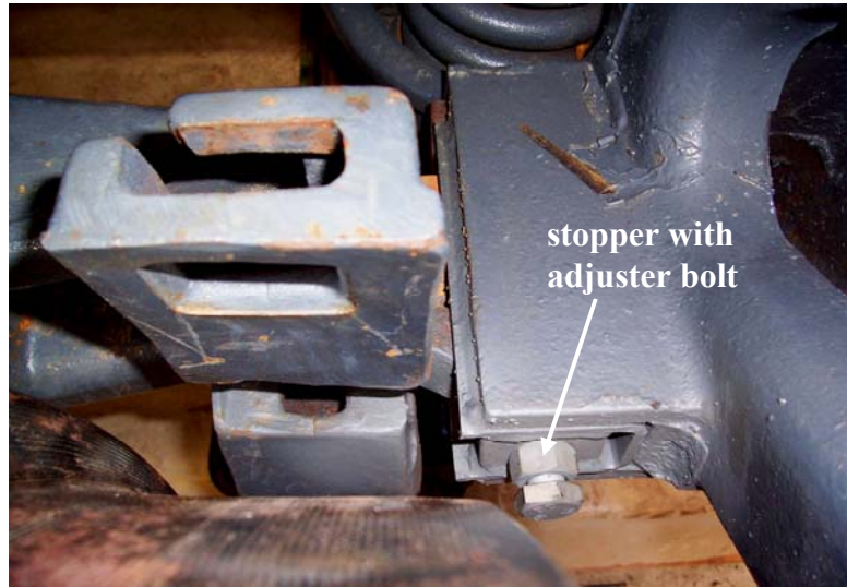
Figure 6.11. Brake beam stopper of the non-braked wheelset
