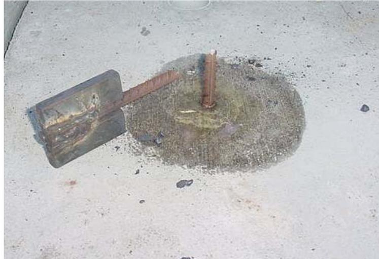
Figure 7.2: Bond test between the new steel bar and the old concrete slab
