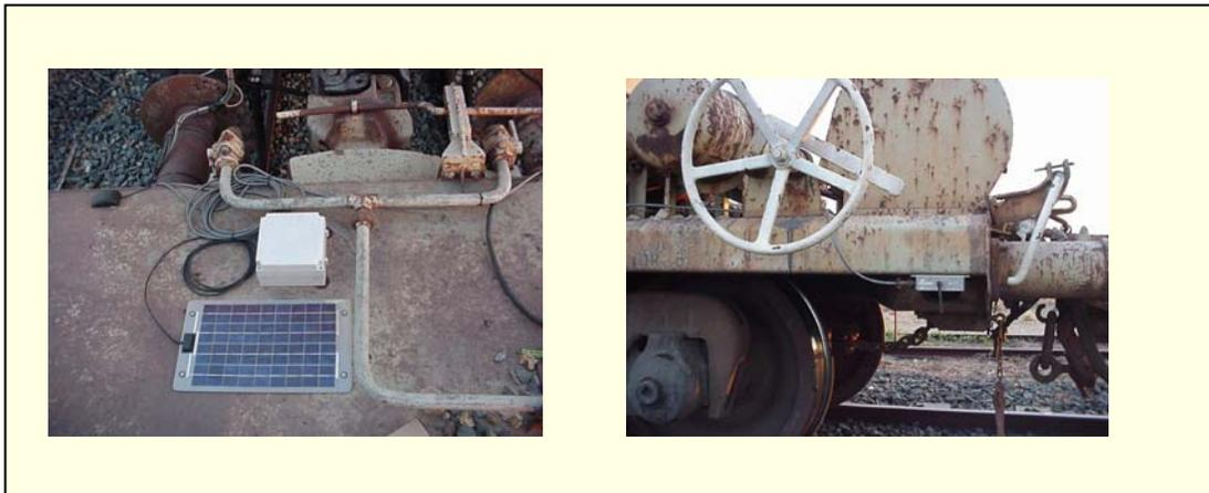
**Figure 3-2 Health Card prototype installed on a ballast wagon**
