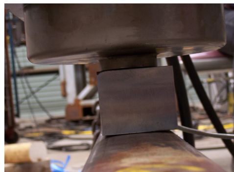
(b) Load transfer to railhead
