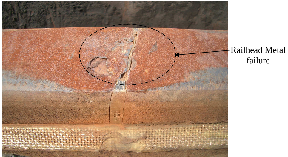
Figure 2.13 Typical IRJ failure in Australian heavy haul networks
